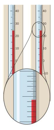
Using the first thermometer, the temperature is 24.3 °C (3 significant digits).
