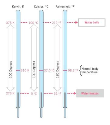
Relationship between the Kelvin (SI), Celsius, and Fahrenheit temperature scales. Kelvin temperature is also called the **absolute temperature** scale.
